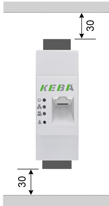
Fig. 5-5: Space requirement, specified in mm
