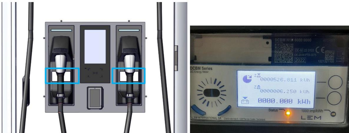
FIGURE 58: DC DISPLAYS ON CHARGING TERMINAL
