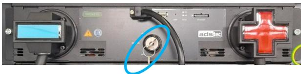
FIGURE 62: SRC4 KEY SWITCH IN "OFF" POSITION
