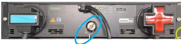
FIGURE 35: SRC4 KEY SWITCH IN "OFF" POSITION
