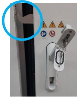
FIGURE 17: ARRESTER HOOK IN POSITION
