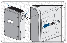
7. Regarding SI4.4M-13: Remove the inverter by lifting it vertically up and off the wall mounting bracket. For this, use the side recess grips. Transport the inverter horizontally.
