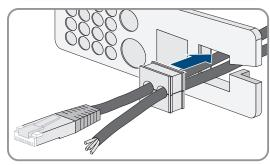
8. Hold the cables and push the cable feed-through plate to the enclosure opening of the cable feed-through plate.
