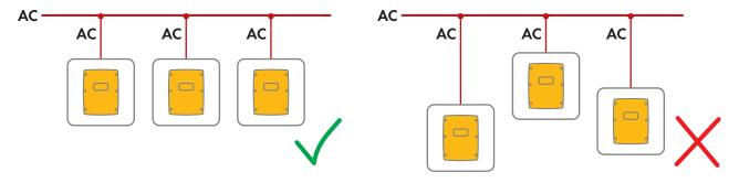
☐ For a single-phase parallel single-cluster system, the cable length and conductor cross-section from each Sunny Island to the AC distribution board must be identical. This will allow for stable and symmetric operation.
