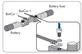
Connect the **BatCur**- insulated measuring conductor on the side for connecting the battery.
