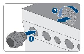
When connecting the cable to connection AC2, attach the M25 cable gland to the AC2 enclosure opening using the counter nut (torque: 7 Nm).
