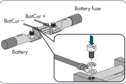
4. Thread both insulated conductors through a ferrite included in the scope of delivery and connect to the terminals **BatCur+** und **BatCur-** on the Sunny Island (see Section 6.6.6, page 61).
