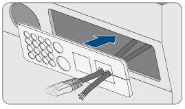
9. Hook the cable feed-through plate into the enclosure opening of the cable feed-through plate and press into the enclosure opening.
