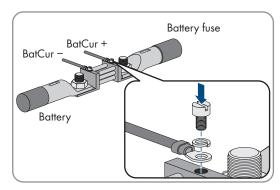
3. Connect the **BatCur-** insulated measuring conductor to the side for connecting the battery on the battery current sensor.
