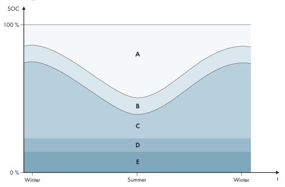
Figure 18: Ranges of the battery state of charge as a function of the season for the northern hemisphere (example)
