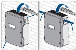
8. Use an Allen key (AF 5) to attach the Sunny Island to the wall mounting bracket on both sides with the M6x10 screws provided (torque: 4 Nm to 5.7 Nm). This will prevent the Sunny Island from being lifted off the bracket.
