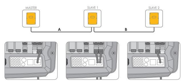
Figure 8: Internal communication cabling (example)
