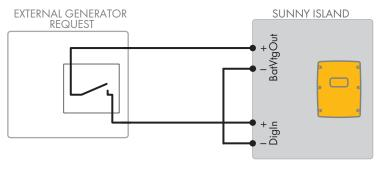
Figure 14: Connection of the control cable of an external generator request (example).
