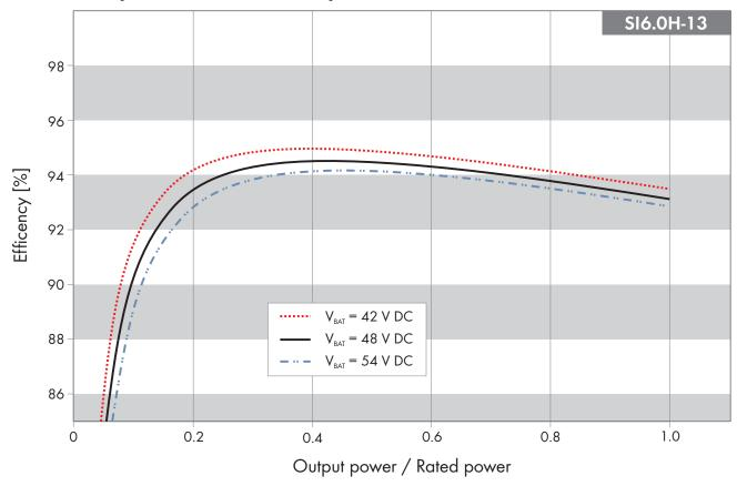
Figure 28: Characteristic efficiency curve
