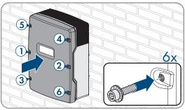
☑ The teeth of the conical spring washer press into the enclosure lid. This ensures that the enclosure lid is grounded.
