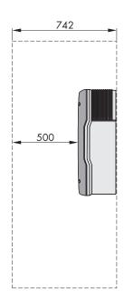
Figure 6: Recommended clearances(Dimensions in mm)
