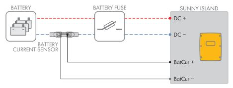
Figure 10: Connection of the battery current sensor to the Sunny Island.
