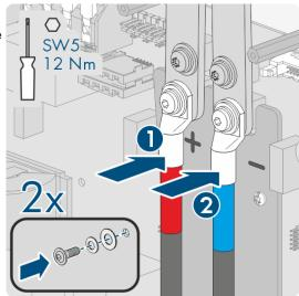
14. Ensure that the entire contact surface of the fender washer is in contact with the terminal lug.
