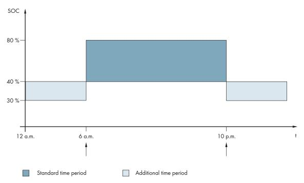
Figure 21: Profile of the SOC thresholds for controlling the load-shedding contactor and the start times for the intervals
