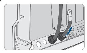
12. Route the **DC**- cable on the side of the protective cover marked with a - symbol.
