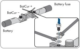
3. Close the battery fuse load-break switch quickly and switch on the Sunny Island.
