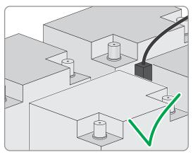
3. Thread both insulated conductors of the sensor through a ferrite included in the scope of delivery and connect to the terminals **BatTmp** on the Sunny Island (see Section 6.6.6, page 61). In this case, the polarity is arbitrary.
