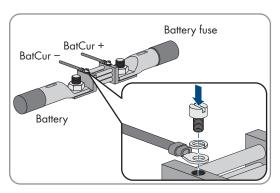
11. Close the battery fuse load-break switch quickly and switch on the inverter.
