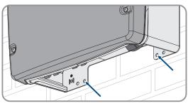
11. Ensure that the Sunny Island is firmly attached.
