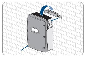
Mount the SI6.0H-13 and SI8.0H-13 to the wall mounting bracket. For this, use the side recess grips or a steel rod (diameter: maximum 30 mm). Keep the Sunny Island in a horizontal position when moving it.
