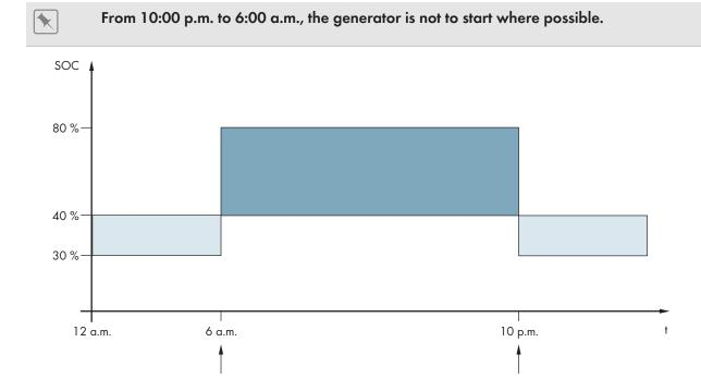
Figure 23: Profile of the SOC and the times for generator requests
