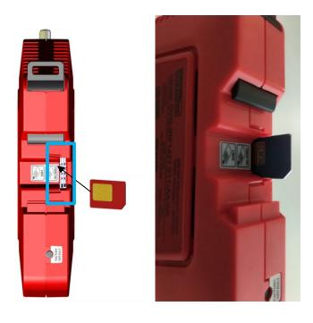
FIGURE 47: INSERTING SIM CARDS INTO THE REAR SIDE OF THE ROUTER
