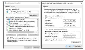
Figure 53: Filling in the network settings on the IPC
