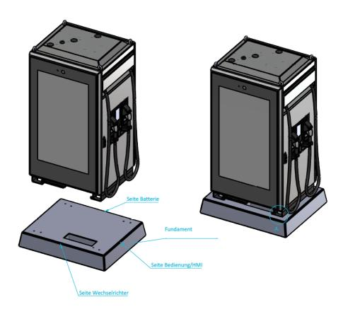
FIGURE 10: PLANNING THE FOUNDATION/FLOOR SPACE FOR THE OVERALL SYSTEM (DETAIL FROM THE CONSTRUCTION DRAWING)
