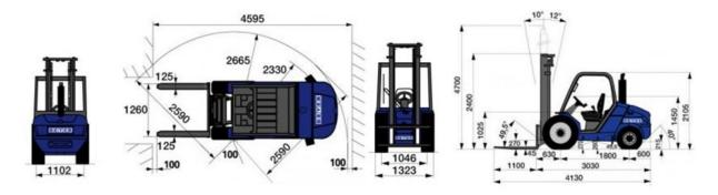
FIGURE 8: MANOEUVRING DIMENSIONS OF A SUITABLE FORKLIFT
