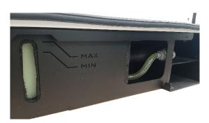
FIGURE 41: COOLANT LEVEL OF THE AIR-CONDITIONING SYSTEM
