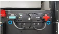
**2** Attach the PE connections at the top of the cover plate.
