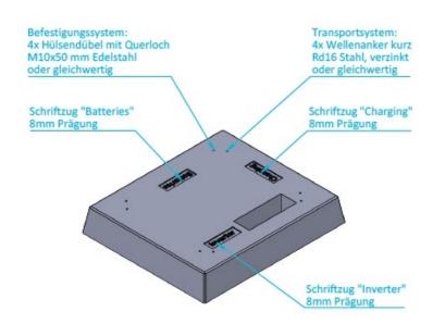
FIGURE 12: EXAMPLE OF A PREFABRICATED FOUNDATION (DETAIL FROM CONSTRUCTION DRAWING)
