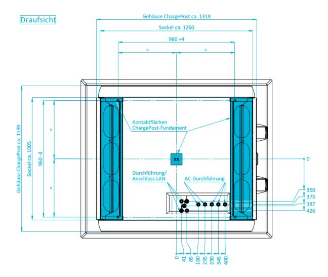
FIGURE 2: SYSTEM DIMENSIONS (TOP VIEW, DETAIL FROM CONSTRUCTION DRAWING)
