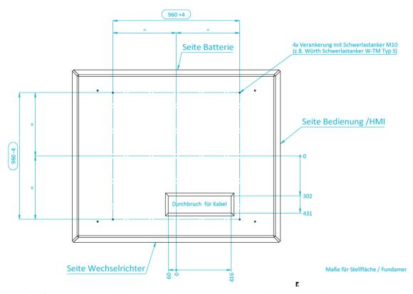
FIGURE 13: DIMENSIONS FOR SCREW CONNECTION TO FLOOR SPACE/FOUNDATION (DETAIL FROM CONSTRUCTION DRAWING)
