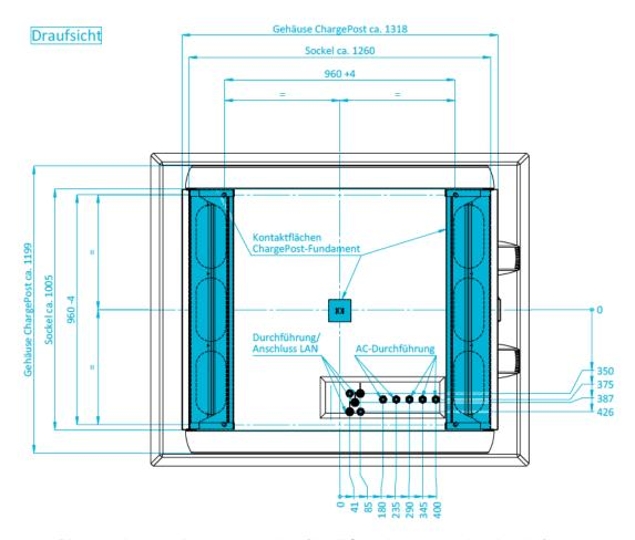
Figure 11: Planning the overall system, top view (detail from the construction drawing)
