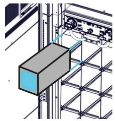
FIGURE 38: BATTERY MODULE INSTALLATION - 1 (EXEMPLARY FIGURE)
