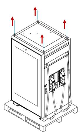
FIGURE 65: LIFTING BY CRANE (DETAIL FROM CONSTRUCTION DRAWING)
