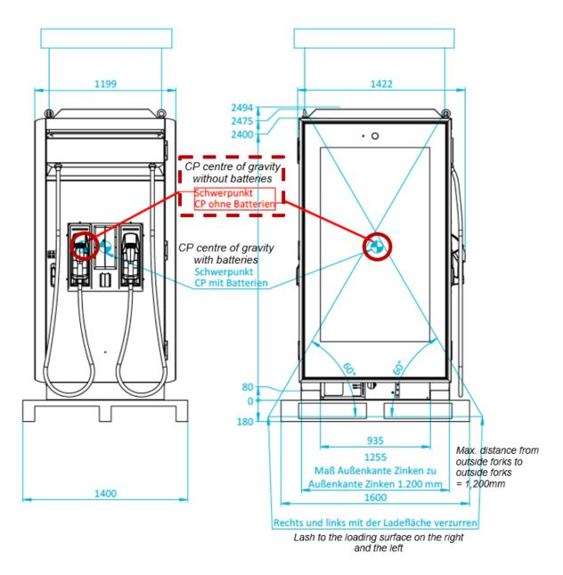
FIGURE 64: CENTRE OF GRAVITY AND DIMENSIONS (DETAIL FROM CONSTRUCTION DRAWING)
