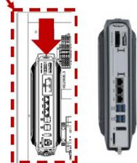
Figure 59: Shutting down IPC using button
