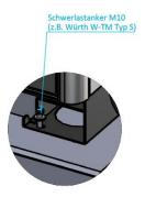
FIGURE 14: SCREW CONNECTION IN DETAIL (DETAIL FROM CONSTRUCTION DRAWING)
