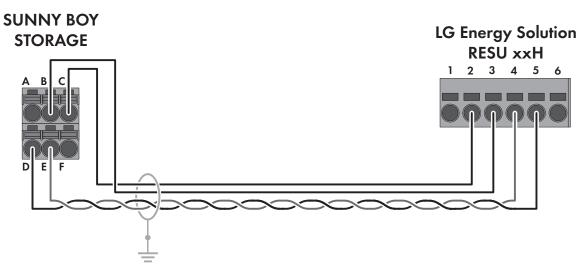
Figure 4: Cabling plan SBS3.7-10 / SBS5.0-10 / SBS6.0-10 with RESU 7H / RESU 10H
