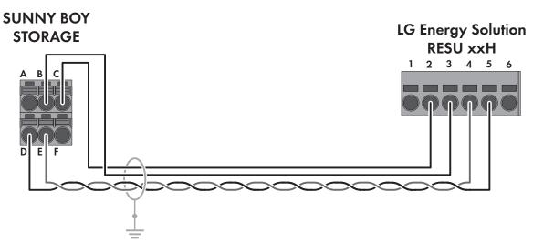
Figure 11: Cabling plan SBS3.8-US-10 / SBS5.0-US-10 / SBS6.0-US-10 with RESU 7H / RESU 10H  $\,$
