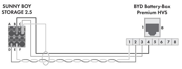
Figure 3: Cabling plan SBS2.5-1VL-10 with Battery-Box Premium HVS
