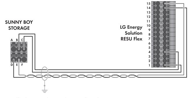
Figure 7: Cabling plan SBS3.7-10 / SBS5.0-10 / SBS6.0-10 with RESU Flex
