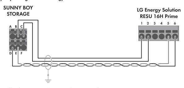
Figure 13: Cabling plan SBS3.8-US-10 / SBS5.0-US-10 / SBS6.0-US-10 with RESU 16H Prime
