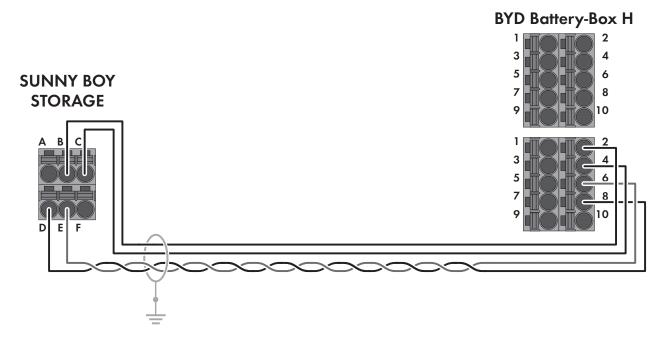
Figure 12: Cabling plan SBS3.8-US-10 / SBS5.0-US-10 / SBS6.0-US-10 with BYD Battery-Box H  $\,$
