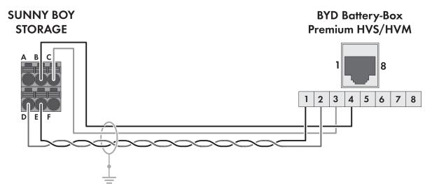
Figure 9: Cabling plan SBS3.7-10 / SBS5.0-10 / SBS6.0-10 with Battery-Box Premium HVS and HVM
