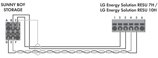
Figure 1: Cabling plan SBS2.5-1VL-10 with RESU  $7\mathrm{H}$  / RESU  $10\mathrm{H}$
