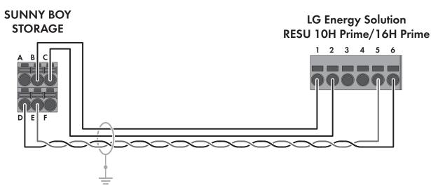
Figure 6: Cabling plan SBS3.7-10 / SBS5.0-10 / SBS6.0-10 with RESU 10H Prime / 16H Prime
