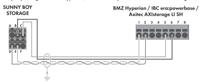
Figure 10: Cabling plan SBS3.7-10 / SBS5.0-10 / SBS6.0-10 with BMZ Hyperion, IBC era:powerbase and Axitec AXIstorage Li SH
